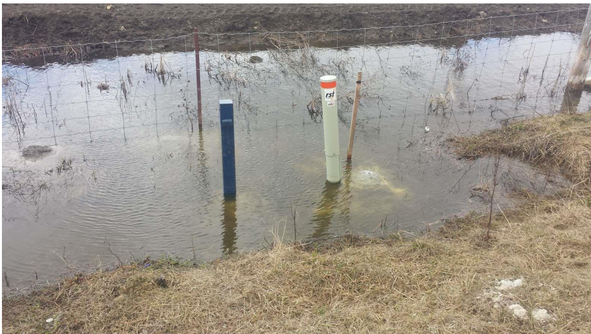
Plate 4: A view of the water ponding along the fenceline at the VWP3 / MW3 pair. The ponding in this area was up to 0.20 m deep (April 10, 2015).
