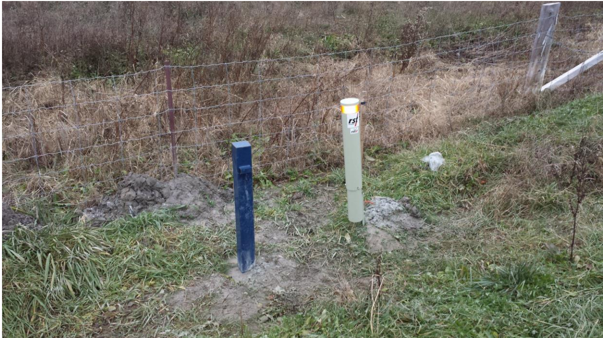
Plate 5: Monitoring well 3 (left) and the pedestal for the vibrating wire piezometer (VWP) 3 datalogger (right) on the west side of the berm (November 26, 2014).
