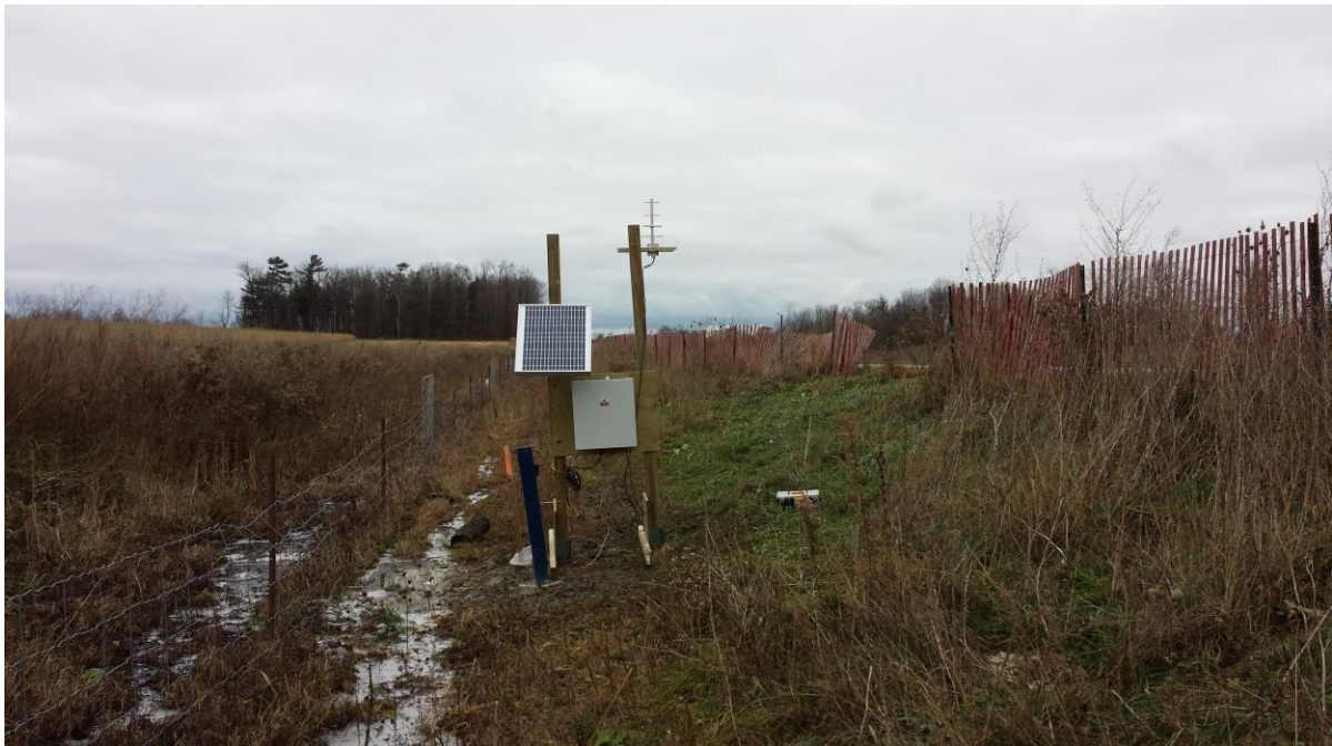
Plate 6: The mounted radio transmission receiver, Flexdaq datalogger, and cellular broadcasting hub at the location of MW5 and VWP5, west of the berm, looking north (November 26, 2014).
