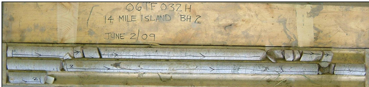
Photograph 1: Cores retrieved from borehole 2. RQD values obtained 76 and 90% for runs 4 and 5 from 1.9 to 4.9 m depth, respectively. Good to excellent rock quality.
