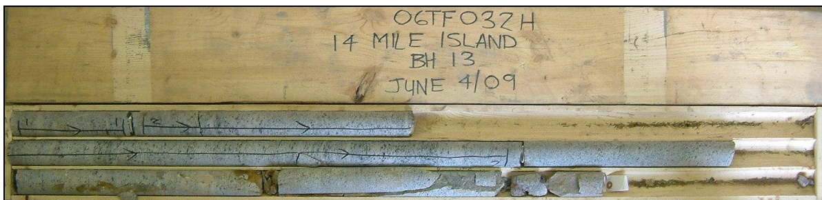
Photograph 8: Cores retrieved from borehole 13. RQD values obtained are 100, 95 and 66% for runs 4 to 6, respectively, from 3.3 to 6.5 m depth, indicating excellent rock quality becoming fair at depth.
