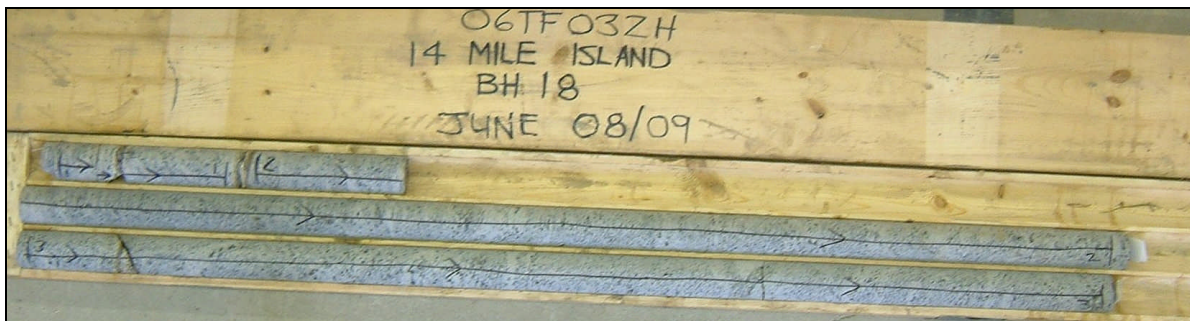
Photograph 11: Cores retrieved from borehole 18. RQD values obtained 67, 100 and 100% for runs 5, 6 and 7, respectively, from 5.2 to 8.5 m depth, indicating fair becoming excellent rock quality.
