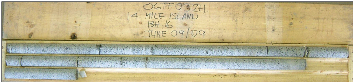
Photograph 10: Cores retrieved from borehole 16. Runs 6 to 8 from 5.0 to 8.2 m depth. RQD values obtained ranged from 94 to 100%, indicating excellent rock quality.
