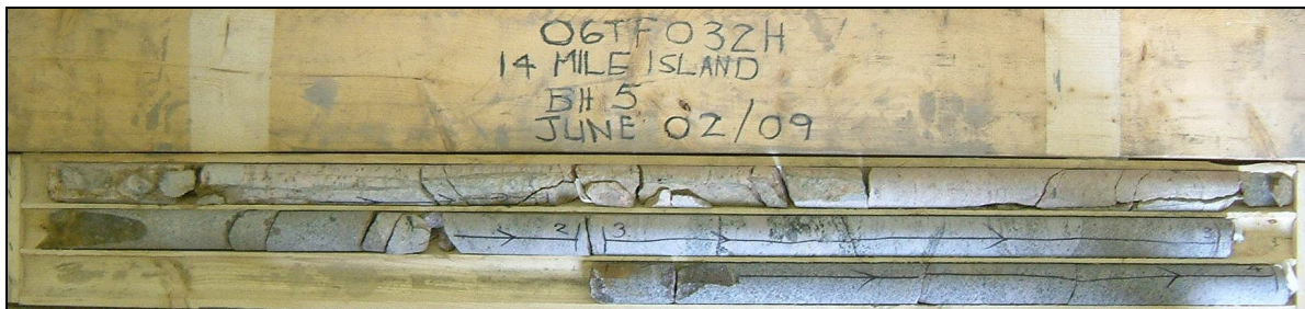
Photograph 3: Cores retrieved from borehole 5. RQD values obtained 65, 41, 100 and 88% for runs 5 to 8, respectively, from 2.8 to 6.4 m depth, indicating poor to fair becoming good to excellent rock quality.
