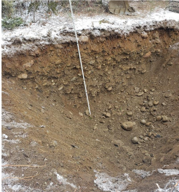
Photo 3. Open test pit to about 3.5 m depth (2018/11/29)
