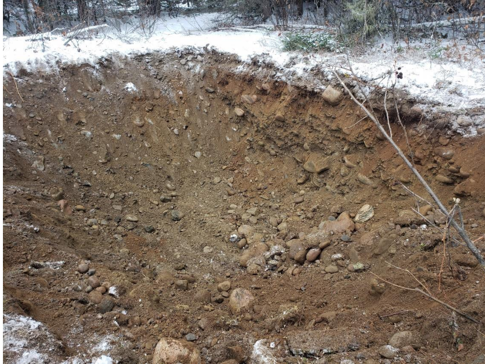
Photo 1. Open test pit to about 2.5 m depth (2018/11/29)
