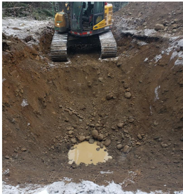
Photo 4. Open test pit to about 3.9 m depth (2018/11/29)
