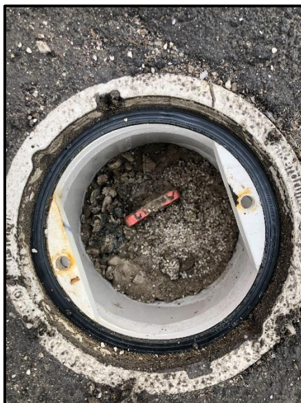
Photograph 3 – Frozen soil/bentonite surrounding an covering plug in piezometer at Borehole CR4-07
