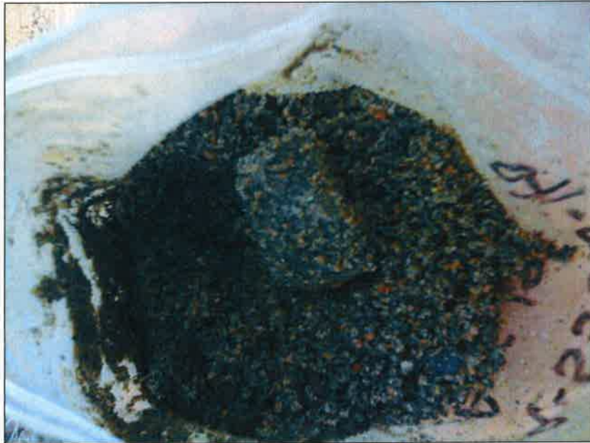
Photograph 6 - Sample from Borehole PINE-03, Run 3, Depth: 18.9 m to 20.4 m depth Soil description: Sand and gravel with cobbles. Cobble diameter: 75 mm
