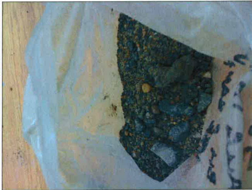
Photograph 5 - Sample from Borehole PINE-03, Run 2, Depth: 17.4 m to 18.9 m. Soil description: Sand and gravel with cobbles. Cobble diameter: 75 mm
