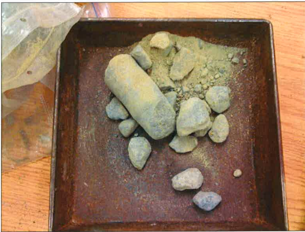
Photograph 7 - Sample from Borehole PINE-03, Run 4, Depth: 20.4 m to 21.9 m Soil description: Sand and gravel with cobbles Cobble diameter: 75 mm to 120 mm
