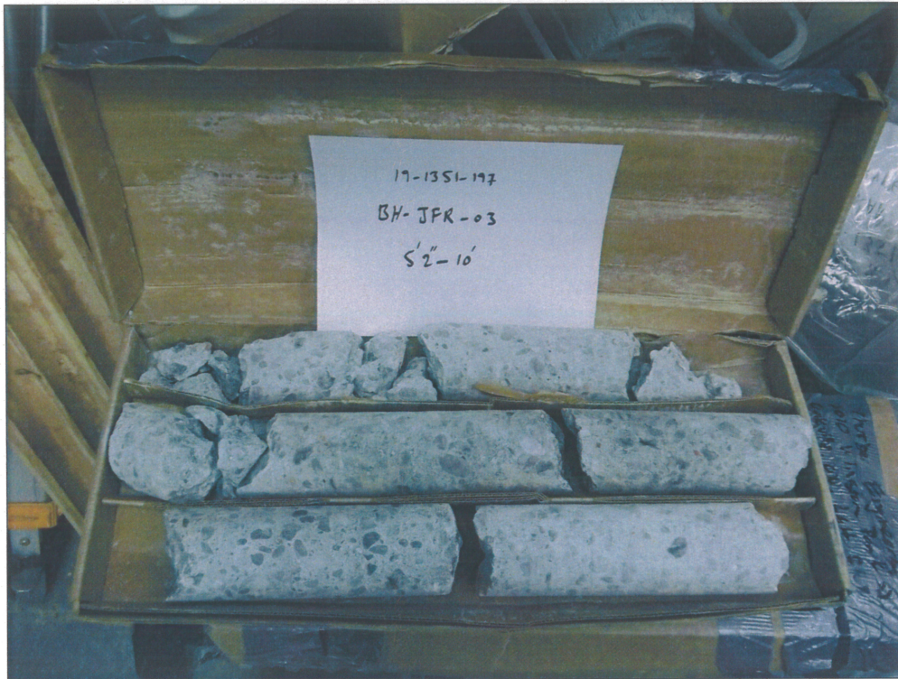
Photograph 2C – Concrete cores, Borehole JFR-03, 1.6 m to 3.0 m depth
