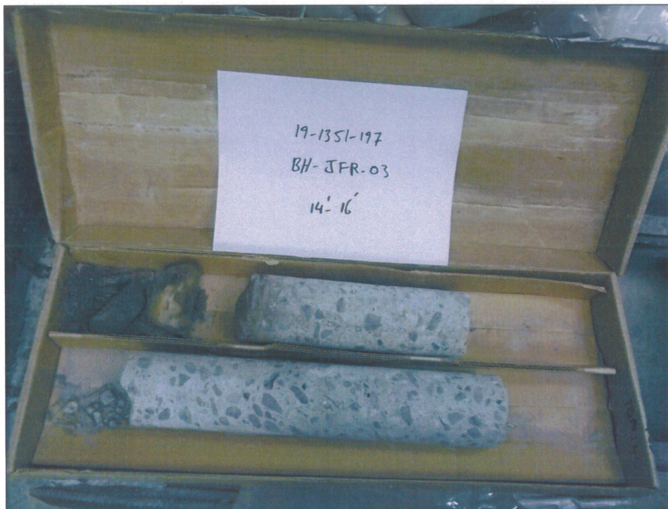
Photograph 4C – Concrete cores, Borehole JFR-03, 4.2 m to 4.9 m depth
