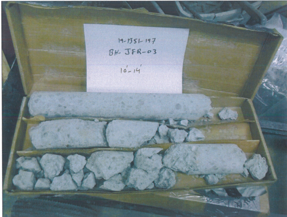
Photograph 3C – Concrete cores, Borehole JFR-03, 3.0 m to 4.2 m depth
