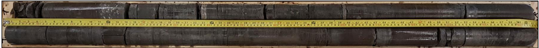
Photograph 4: Cores retrieved from borehole BH-4. Runs 2 and 3 from 9.8 to 12.9 m depth. RQD values ranged from 86 to 91%, indicating good to excellent rock quality.
