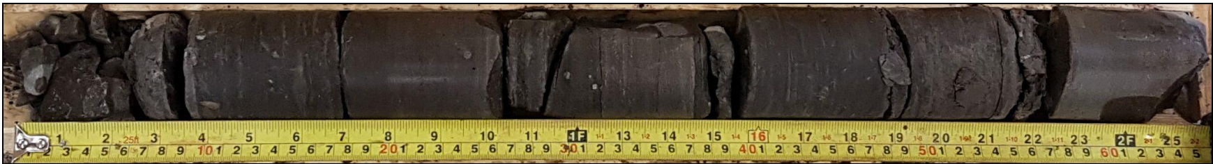
Photograph 3: Core retrieved from borehole BH-4. Run 1 from 9.2 to 9.8 m depth. RQD value was 10%, indicating very poor quality.
