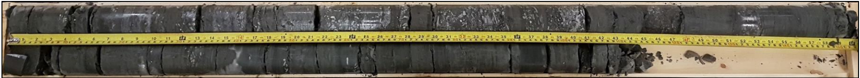
Photograph 1: Cores retrieved from borehole BH-1. Runs 1 and 2 from 12.8 to 15.4 m depth. RQD values ranged from 11 to 79%, indicating very poor to good rock quality.
