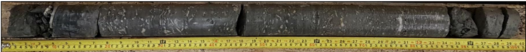
Photograph 2: Core retrieved from borehole BH-1. Run 3 from 15.4 to 16.4 m depth. RQD value was 73%, indicating fair quality.
