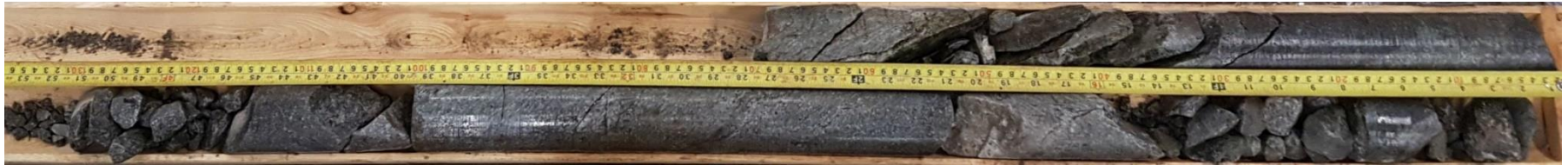
Photograph 3: Borehole DC-3, Runs 1 and 2.
