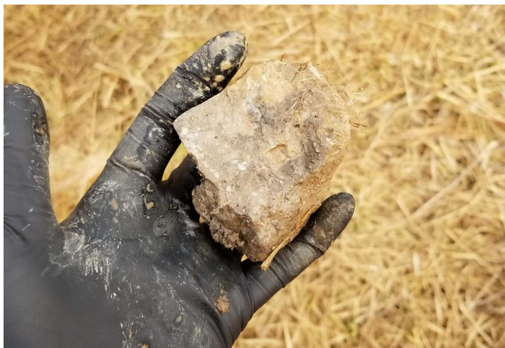
Photograph 1: Large gravel-sized particle from cuttings of Borehole 326-4
