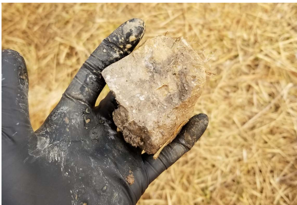
Photograph 1: Large gravel-sized particle from cuttings of Borehole 326-4
