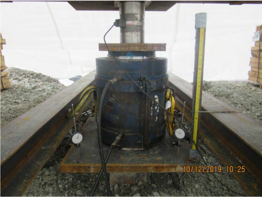
Photograph 14: Load Cell and Jack Setup
