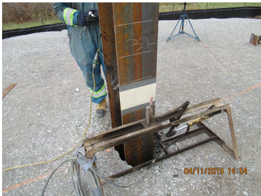
Photograph 8: Setup of Hiley Test and PDA Test Equipment
