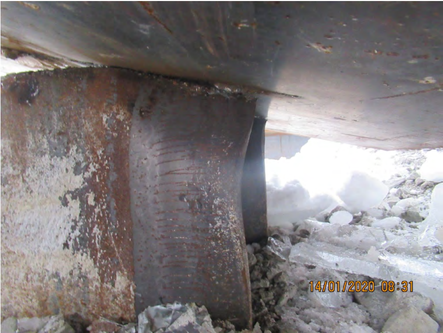
Photograph 2: Test Pile upon Failure during Procedure B Static Pile Load Test
