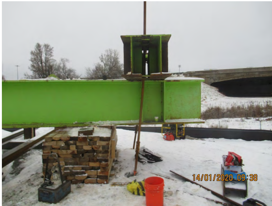
Photograph 3: Reaction pile lateral movement (south side).
