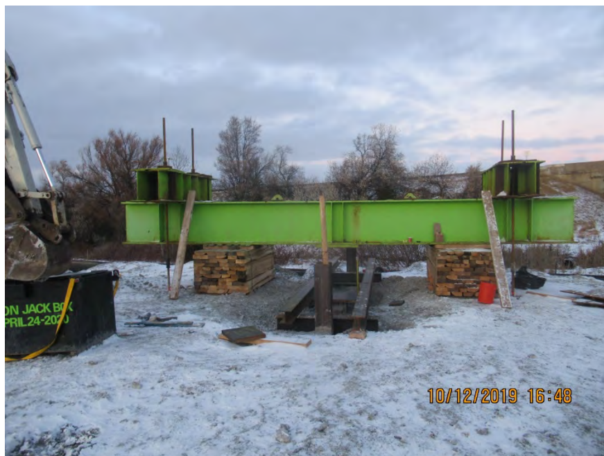
Photograph 12: Reaction Frame with Test Pile Cut to Below Existing Ground Surface
