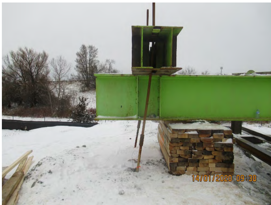
Photograph 4: Reaction pile lateral movement (north side)
