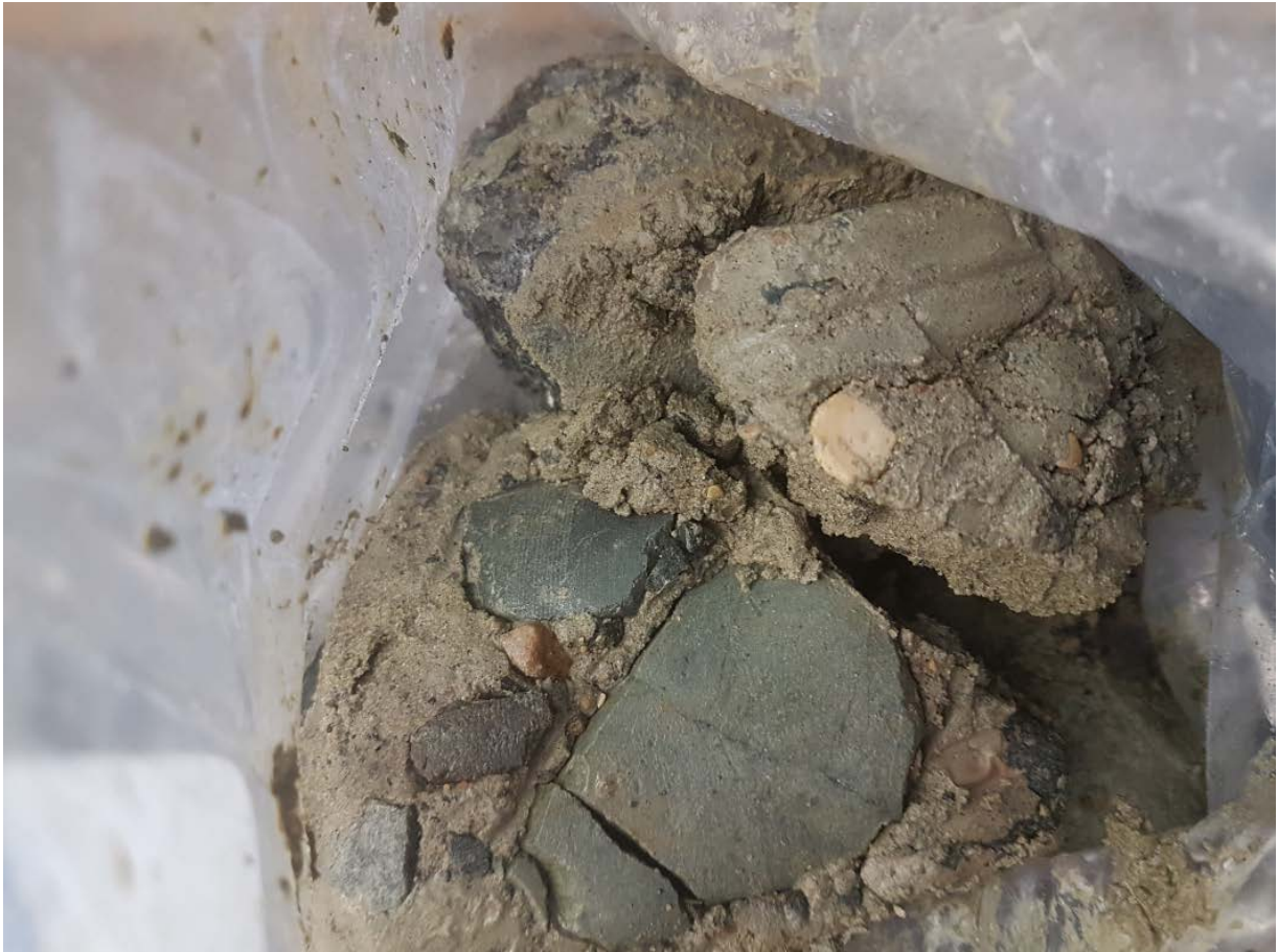
Photograph P4 – Cobbles and Gravel within the Sand to Silty Sand Deposit in Borehole 17-3.
