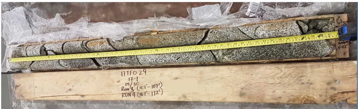
Photograph P8 – A Rock Core from Borehole 17-1 at a Depth of 31 m (102 ft.)
