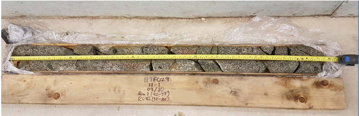
Photograph P7 – A Rock Core from Borehole 17-1 at a Depth of 28 m (92 ft.).
