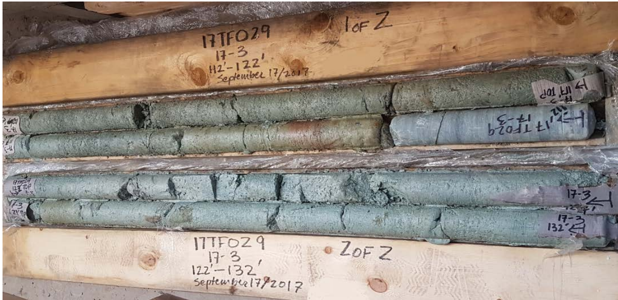
Photograph P5 – Sandy Silt Till Cores Retrieved from Borehole 17-3. Note the Granite/Granodiorite Boulder at a Depth of about 36 m (118 ft.).
