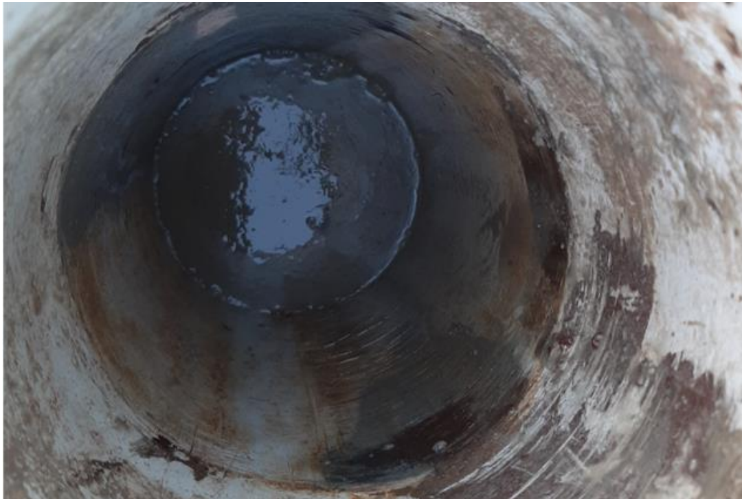
Photograph 8 - The Groundwater Level inside the Riser Pipe at Borehole 35-617-10
