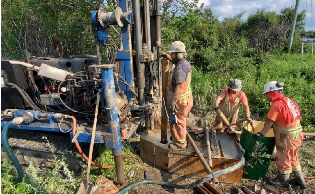
Photograph 7 - Measuring Artesian Head in a Riser Pipe at Borehole 35-617-10
