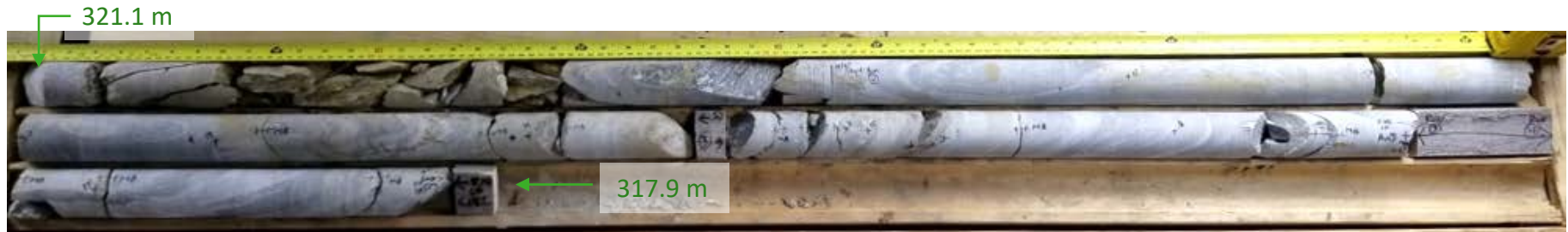
Borehole NR-3 Elevation 321.1 m to 317.9 m
