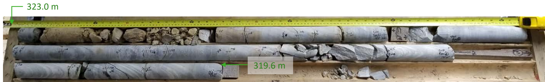
Borehole NR-1 Elevation 323.0 m to 319.6 m
