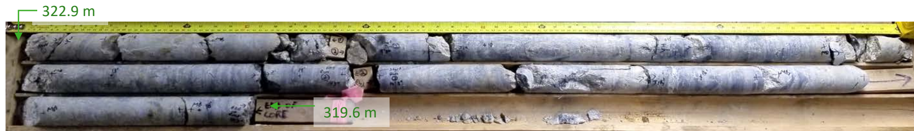
Borehole NR-6 Elevation 322.9 m to 319.6 m
