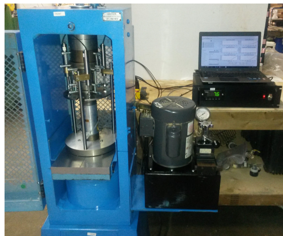
Figure 1: Forney loading frame setup for UCS testing.
