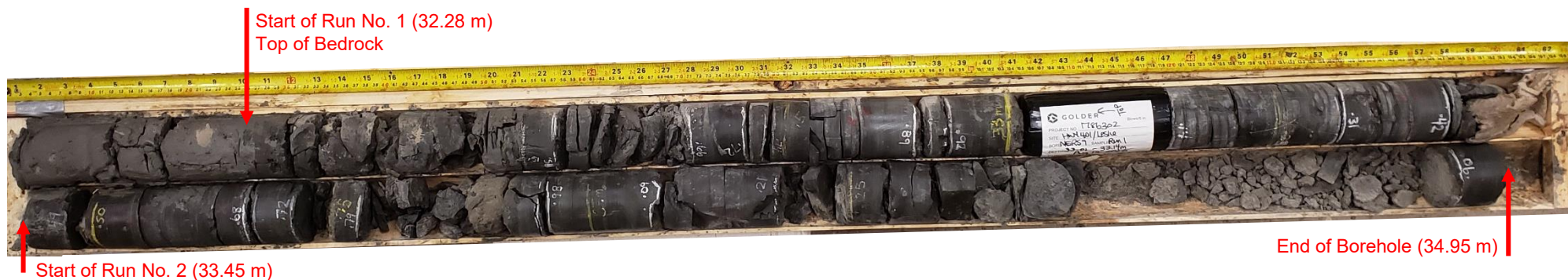
Borehole N/E RS-9: Bedrock cored between depths of about 32.28 m to 34.95 m
