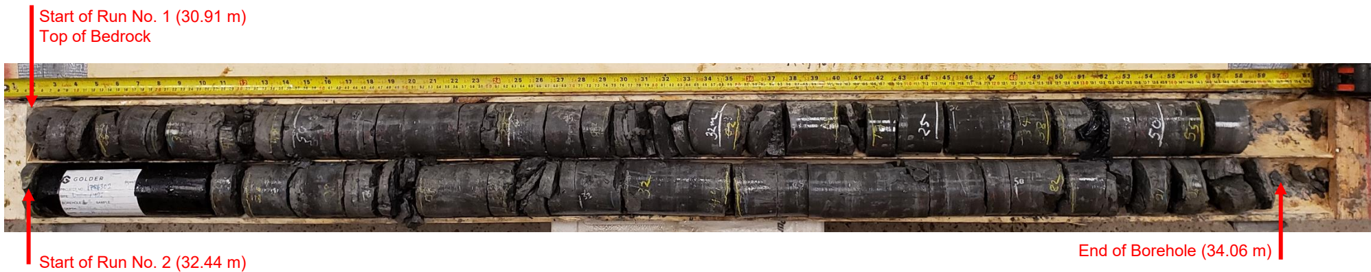
Borehole L-3: Bedrock cored between depths of about 30.91 m to 34.06 m
