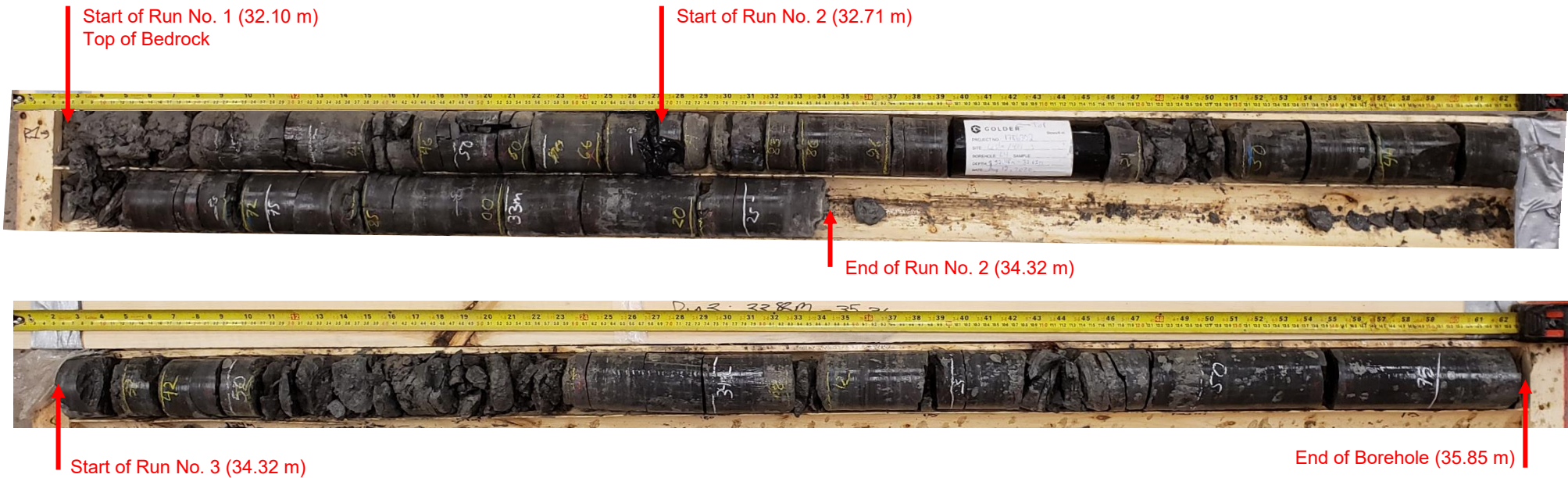
Borehole L-4: Bedrock cored between depths of about 32.10 m to 35.85 m
