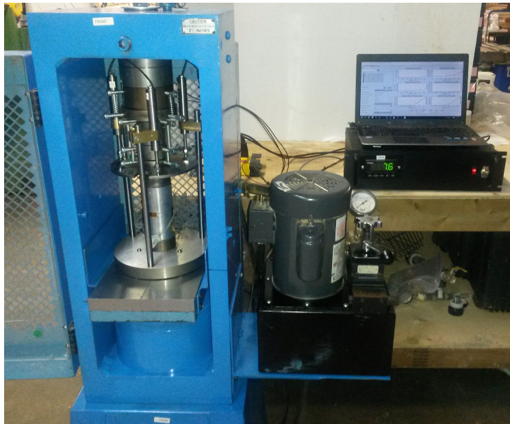
Figure 1: Forney loading frame setup for UCS testing.
