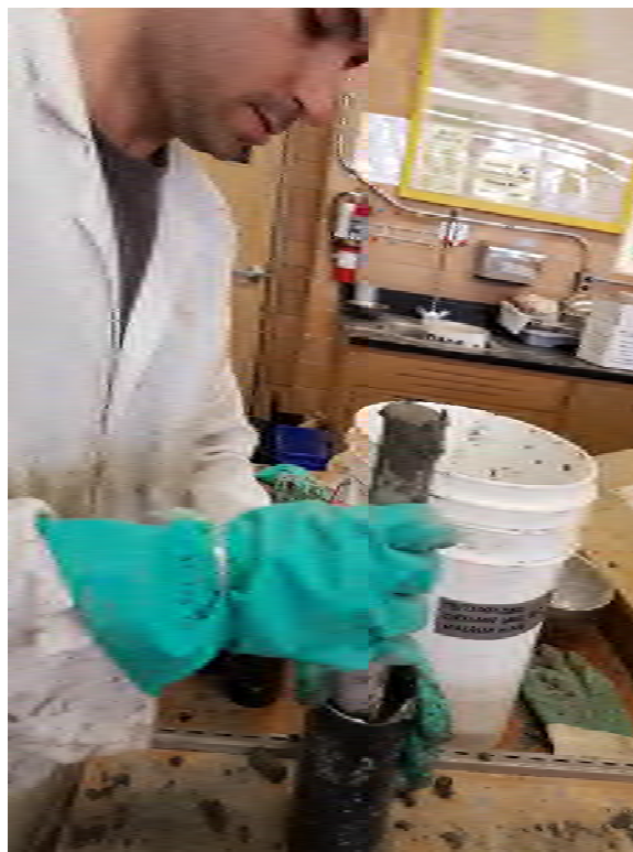
Figure 2.4. Picture of compacting the mixture into the plastic mold
