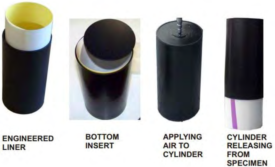
Figure 2.2. Reusable plastic mold used for sample curing (Deslauries, 2017)
