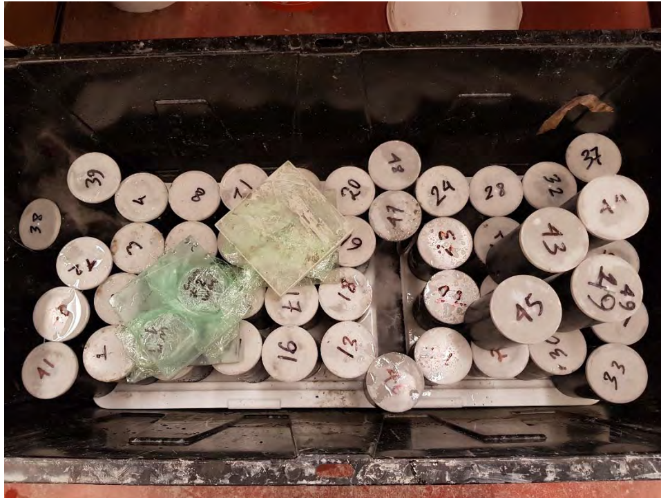
Figure 2.5. Picture of samples numbered and put in the humid chamber for curing
