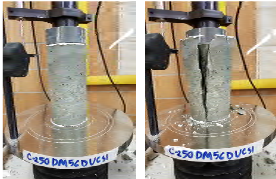
Figure 4.2 A typical UCS test on a dry mixing sample before and after failure
