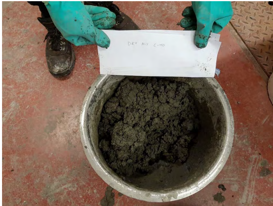
Figure 2.3. Picture of soil and cement after dry mixing
