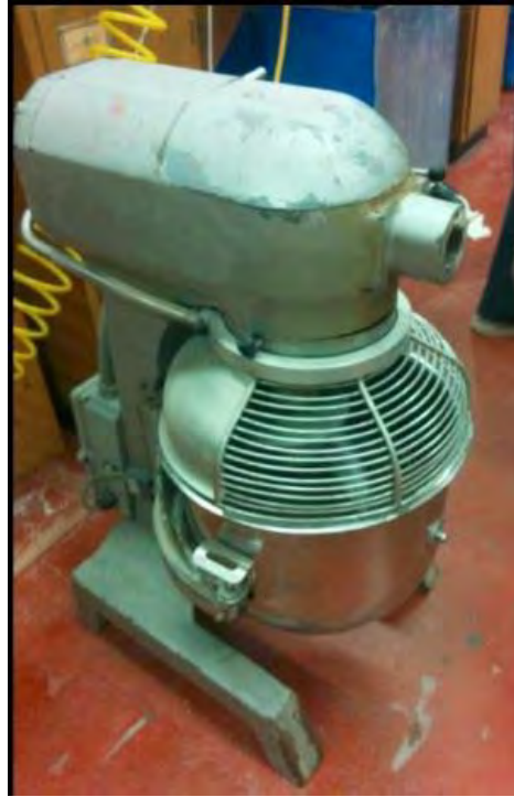
Figure 2.1. Hobart A200 mixer used for soil mixing
