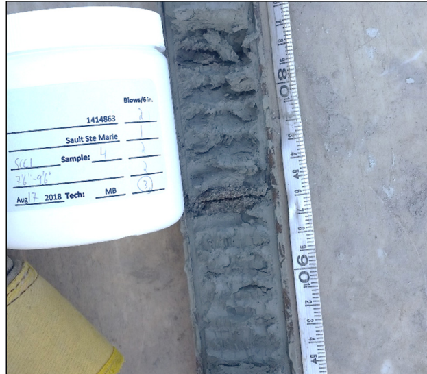
Photograph 6: Silt to clayey silt laminae (light grey colour) and silty clay laminae (dark grey colour)
