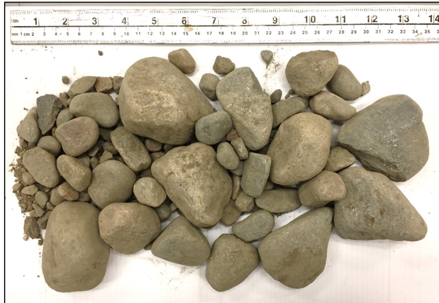
Photograph 5: Cobbles and rock fragments – auger sample recovered from the upper portion of the embankment fill (in Borehole SCC-02) where difficulty with auger advancement was encountered.
