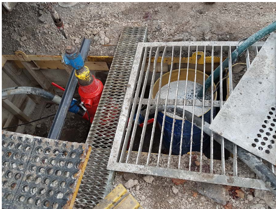
Photograph 7: Blow-out prevention system on the borehole
