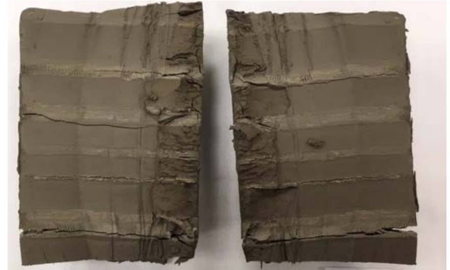
Photograph 2: Soil Sample from Borehole 89UP-07 Sample 21 (Location of Proposed East Abutment)
