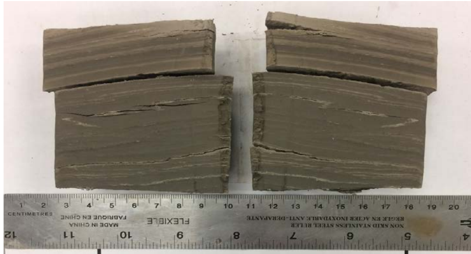
Photograph 1: Soil Sample from Borehole 89UP-03 Sample 20 (Location of Proposed West Abutment)
