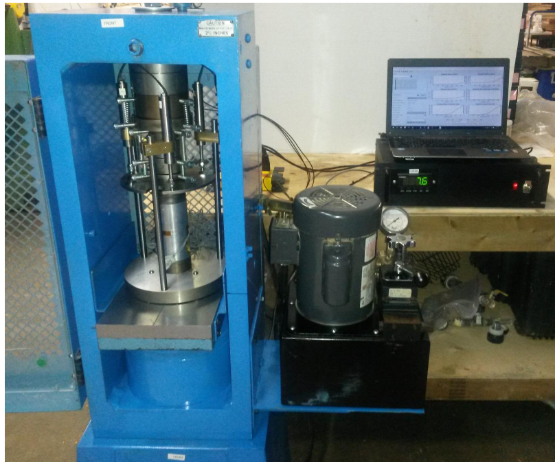
Figure 1: Uniaxial Compressive Strength (UCS) test setup.
