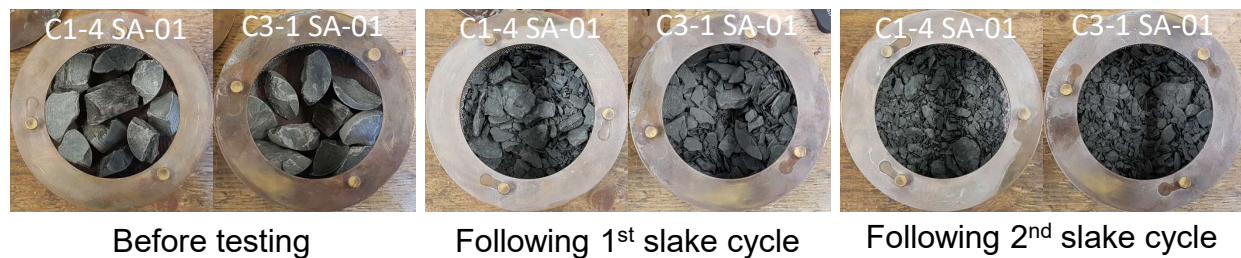
Figure 7: Photographs of slake durability specimens before and after testing.
