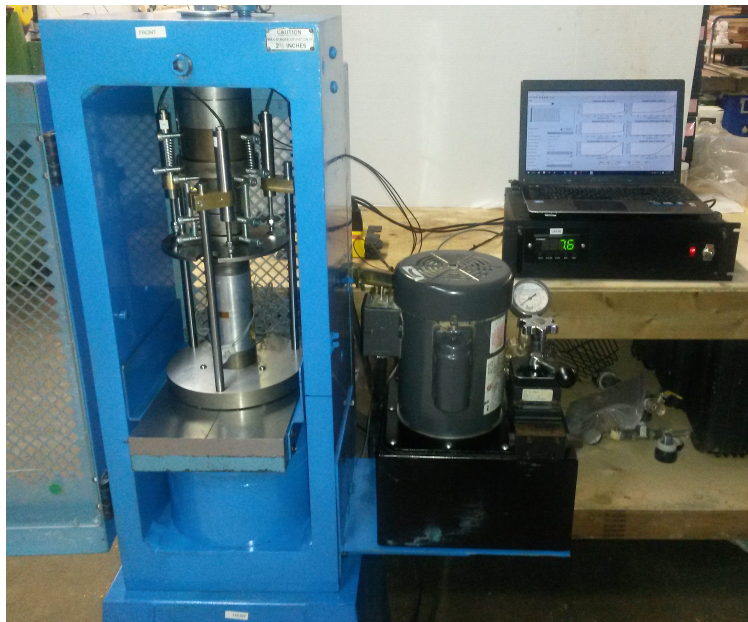
Figure 1: UCS test setup.
