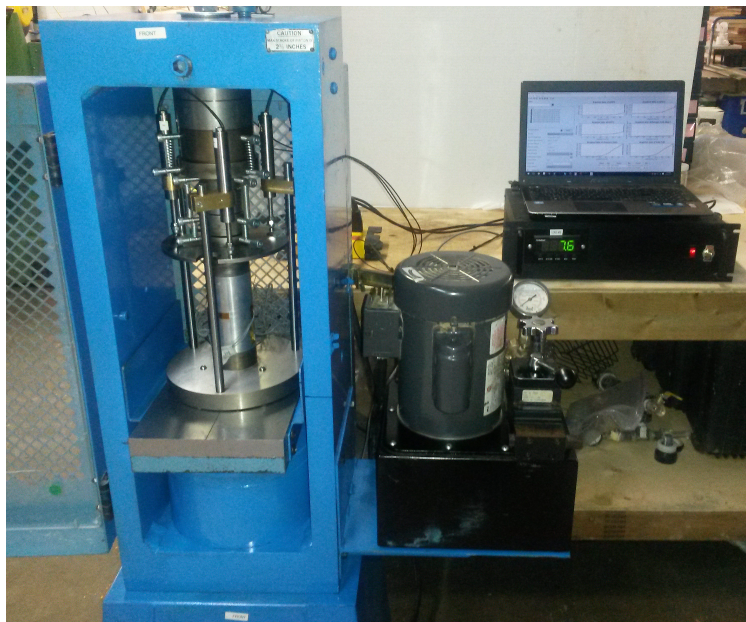
Figure 1: UCS test setup.
