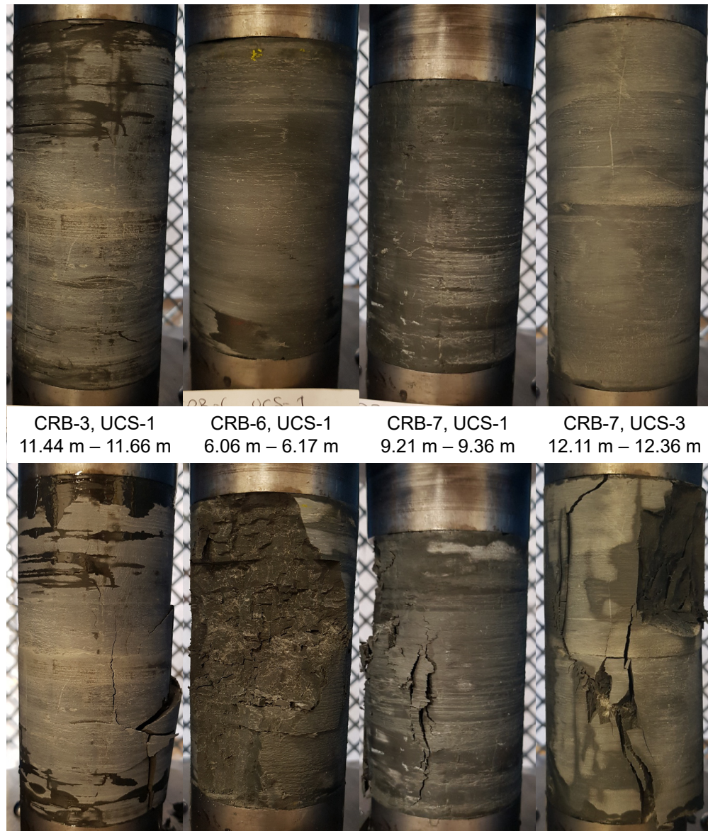
Figure 3: Photographs of specimens prior to testing.
