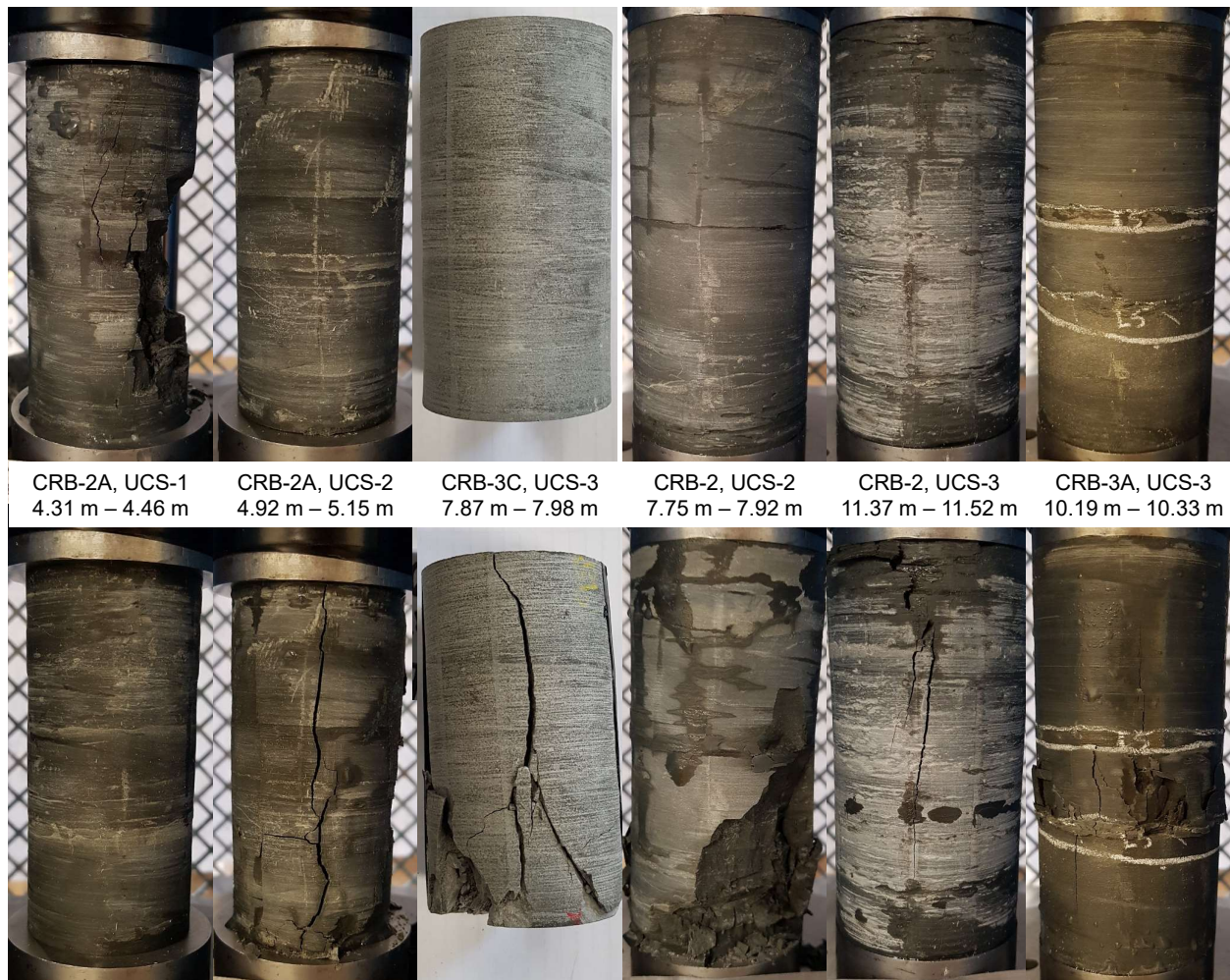
Figure 3: Photographs of specimens prior to testing.
