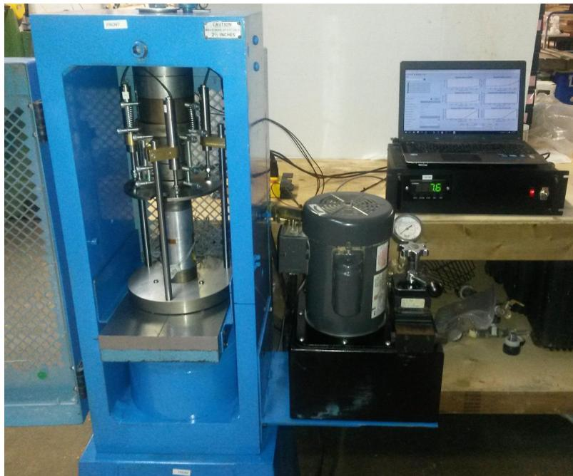
Figure 1: UCS Test setup.
