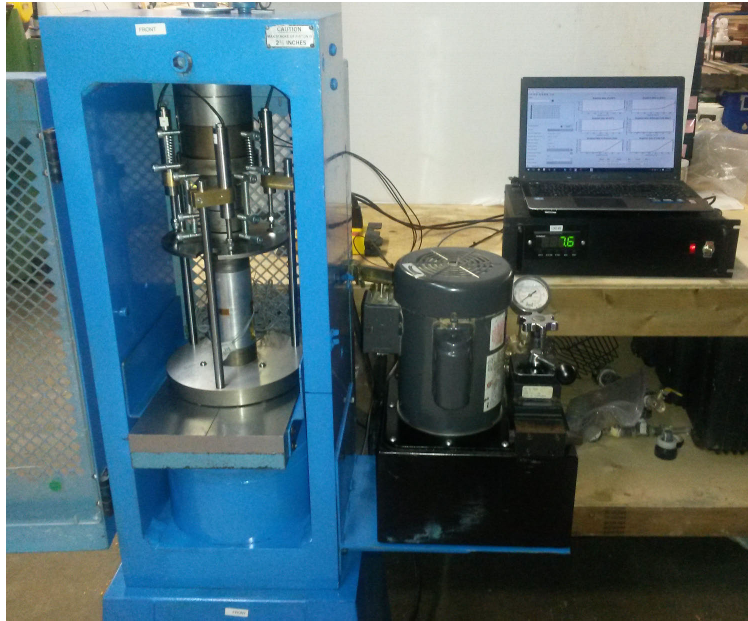
Figure 1: Forney loading frame setup for uniaxial compression testing.
