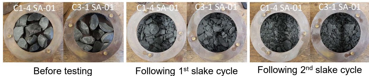
Figure 7: Photographs of slake durability specimens before and after testing.
