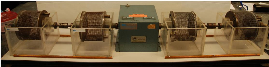
Figure 6: Test setup showing the slake durability apparatus.
