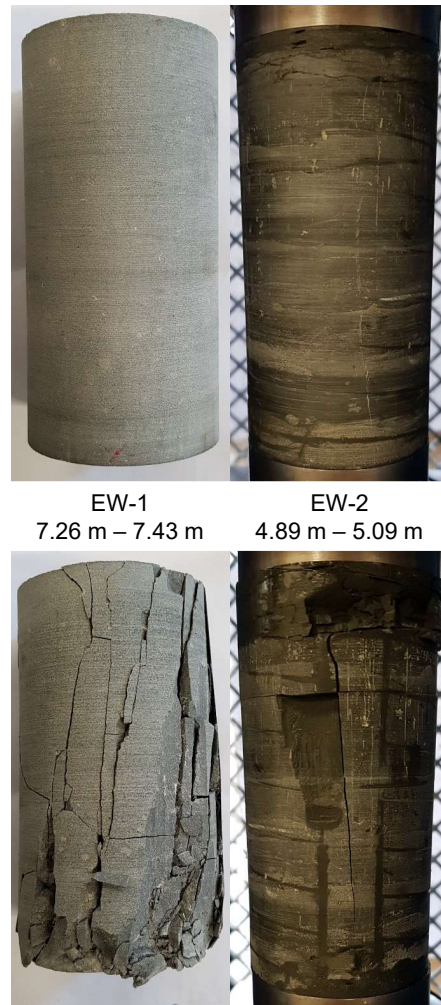
Figure 3: Photographs of specimens before and after testing.
