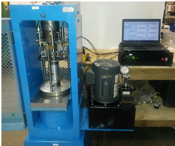
Figure 1: UCS test setup.
