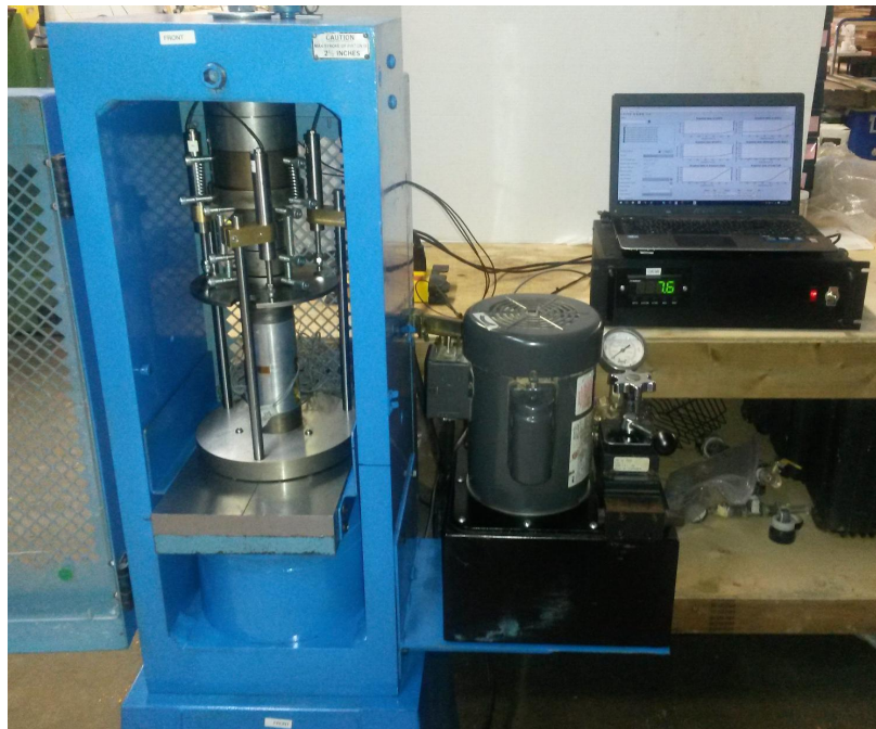
Figure 1: UCS Test setup.
