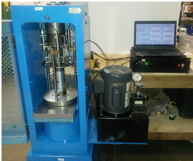
Figure 1: UCS test setup.
