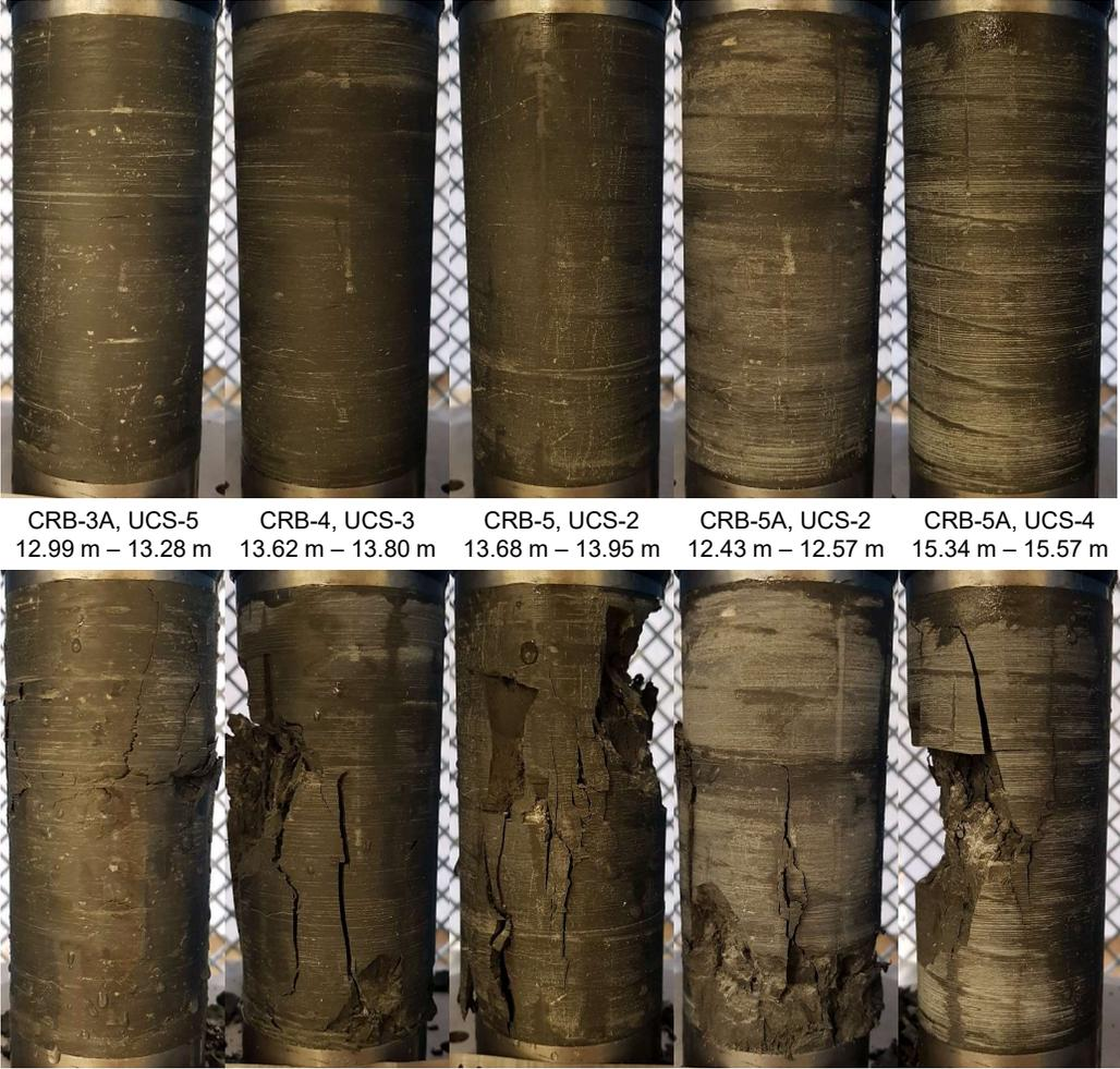
Figure 4: Photographs of failed specimens after testing.
