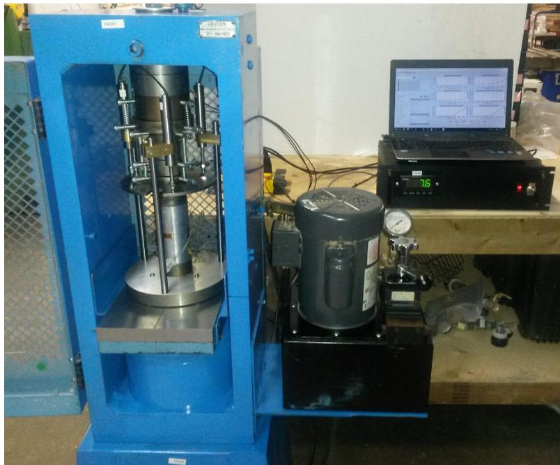
Figure 1: UCS Test setup.
