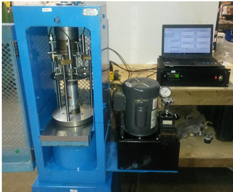
Figure 1: UCS test setup.
