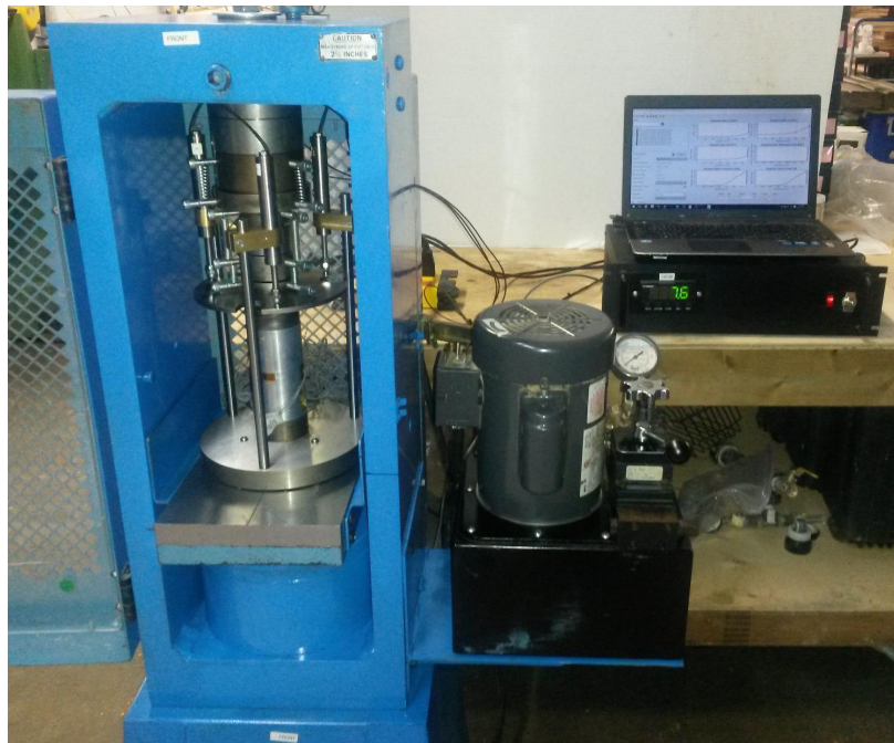
Figure 1: UCS Test setup.
