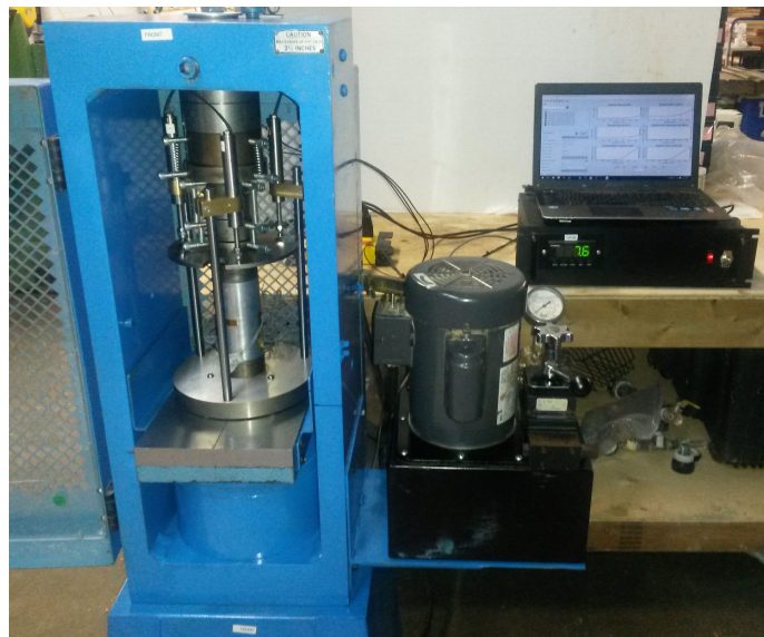
Figure 1: Forney loading frame setup for UCS testing.
