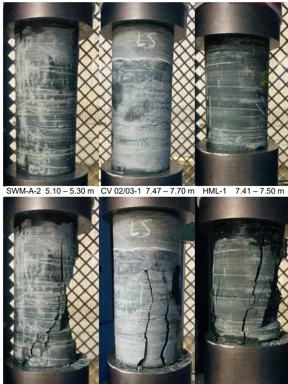
Figure 3: Photographs of test specimens before testing (top) and after testing (bottom).
