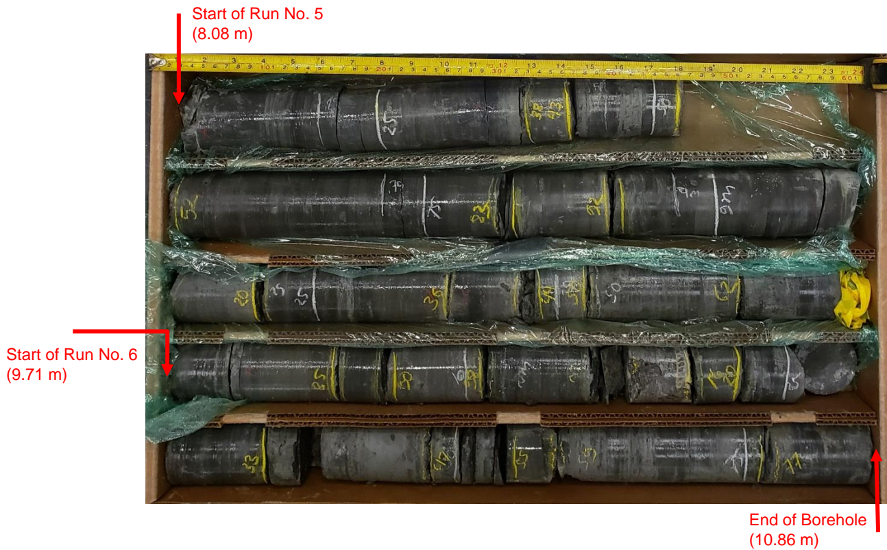
Borehole 21-35: Bedrock cored between depths of about 8.08 m to 10.86 m
