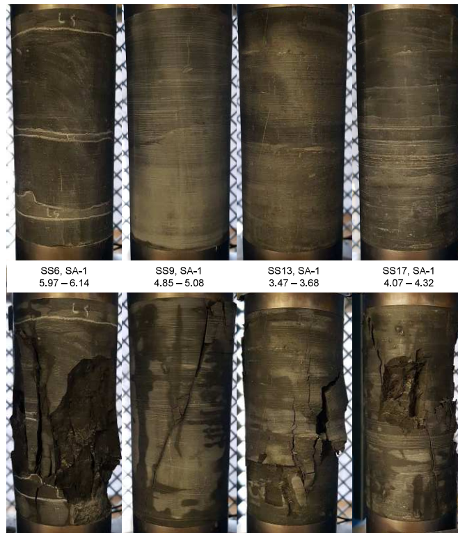
Figure 4: Photographs of UCS specimens before testing (top) and after testing (bottom).
