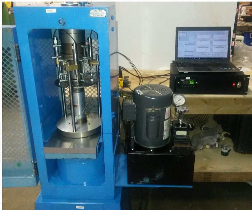
Figure 1: Equipment setup for measuring Uniaxial Compression Strength (UCS).
