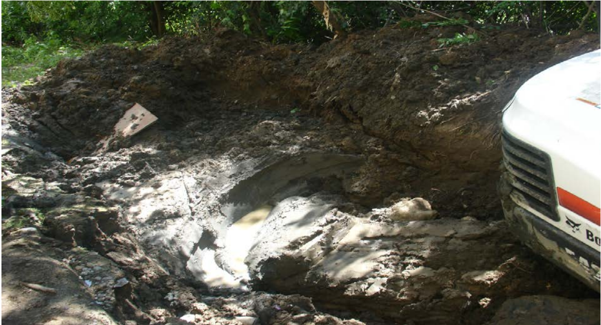
Photograph 5: Surface soil was very soft and swampy, silty sand layer was saturated by water leaking from a retaining wall weep hole and stormwater ponding. (July 2015)
