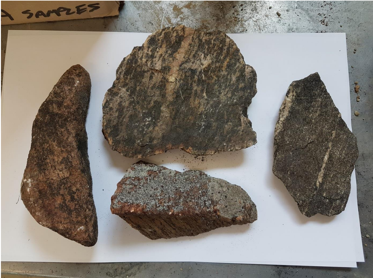
Photograph 5: Rock Samples, chipped by pick axe from the rock out crop found within the proposed culvert footprint.
