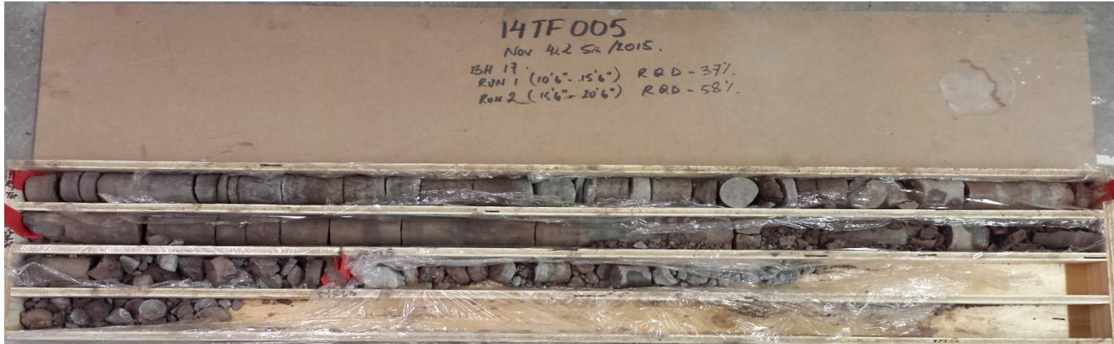
Photograph 3: Cores retrieved from borehole 17. Rock cores 1 to 2 from 3.2 to 6.2 m. RQD values ranged from 37 to 58%, indicating poor to fair rock quality.
