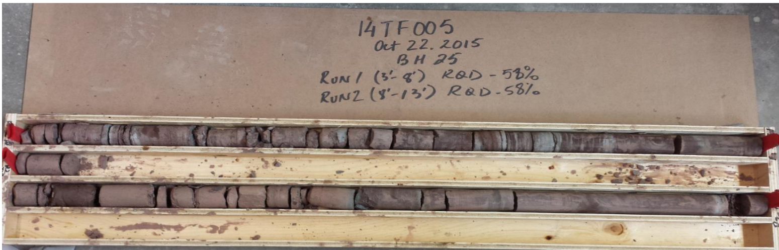
Photograph 4: Cores retrieved from borehole 25. Rock cores 1 to 2 from 0.9 to 4.0 m. RQD values ranged from 52% to 58%, indicating fair rock quality.
