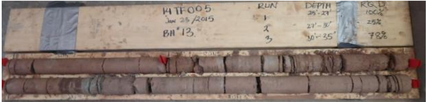
Photograph 1: Cores retrieved from borehole 13. Rock cores 1 to 3 from 7.6 to 10.7 m. RQD values ranged from 25% to 100%, indicating poor to excellent rock quality.
