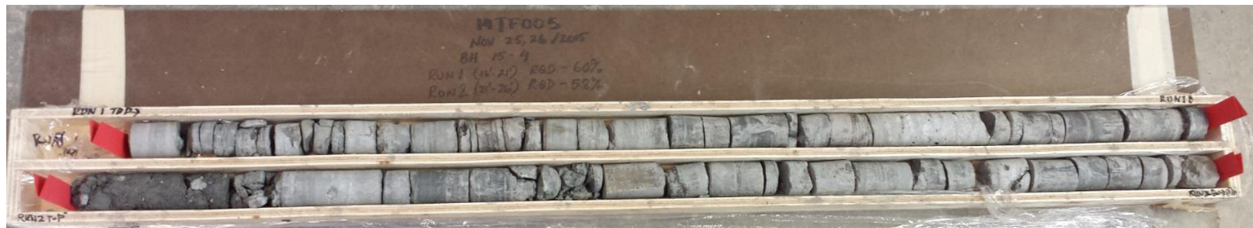
Photograph 2: Cores retrieved from borehole 15-4. Rock cores 7 and 8 from 4.9 to 7.9 m. RQD values were 60% and 58% respectively, indicating fair rock quality.
