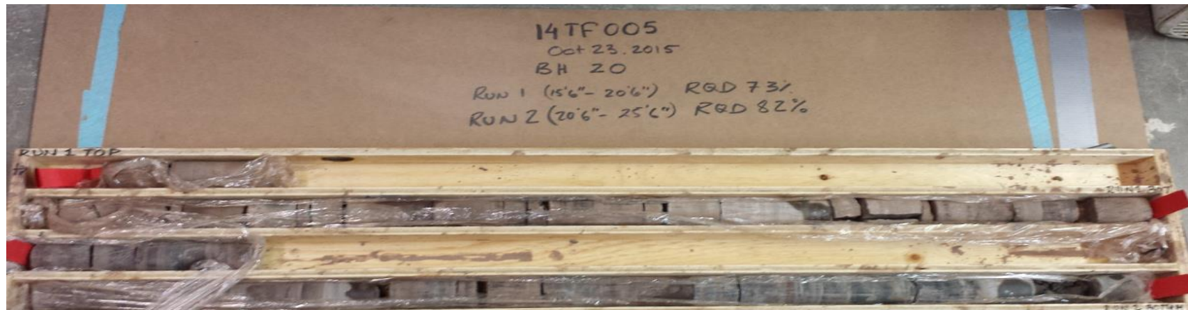
Photograph 1: Cores retrieved from borehole 20. Cores 8 and 9 from 4.7 to 7.8 m depth. RQD values were 73 and 82%, indicating fair to good rock quality.
