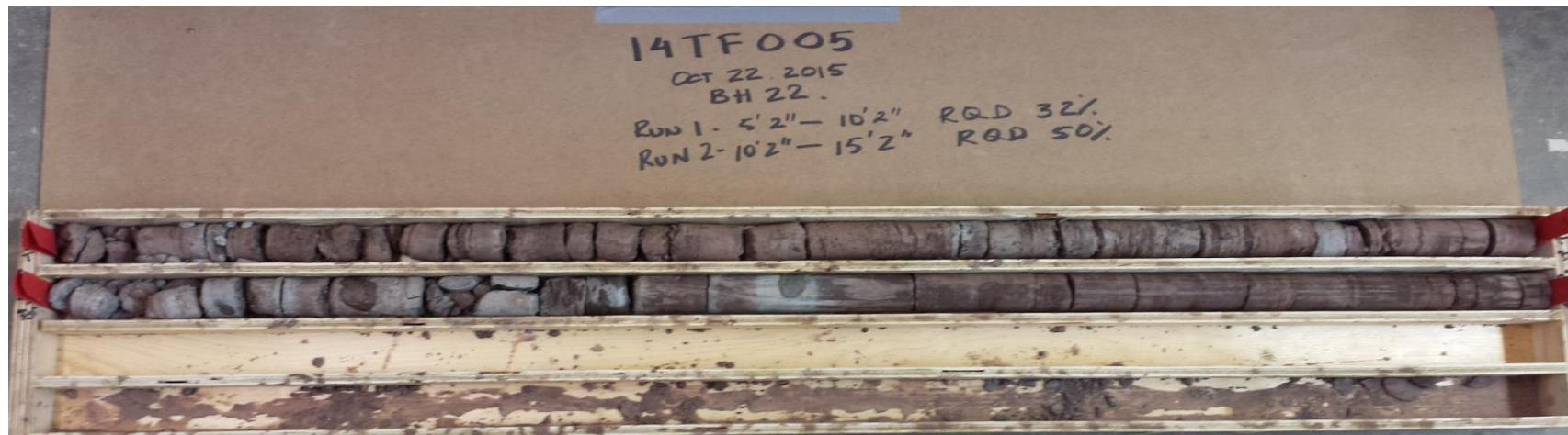
Photograph 2: Cores retrieved from borehole 22. Cores 4 and 5 from 1.6 to 4.6 m depth. RQD values were 32 and 50%, indicating poor to fair rock quality.
