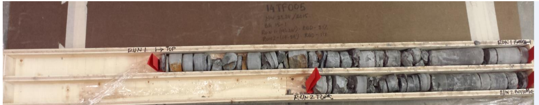
Photograph 1: Cores retrieved from borehole 15-1. Rock cores 7 and 8 from 5.8 to 8.8 m. RQD values ranged were 31% and 11% respectively, indicating poor to very poor rock quality.
