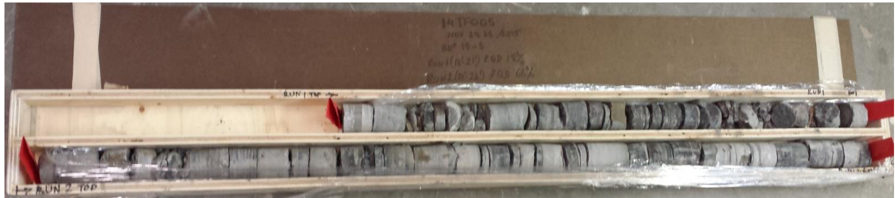
Photograph 2: Cores retrieved from borehole 15-3. Rock cores 7 and 8 from 4.9 to 7.9 m. RQD values were 18% and 67% respectively, indicating very poor to fair rock quality.
