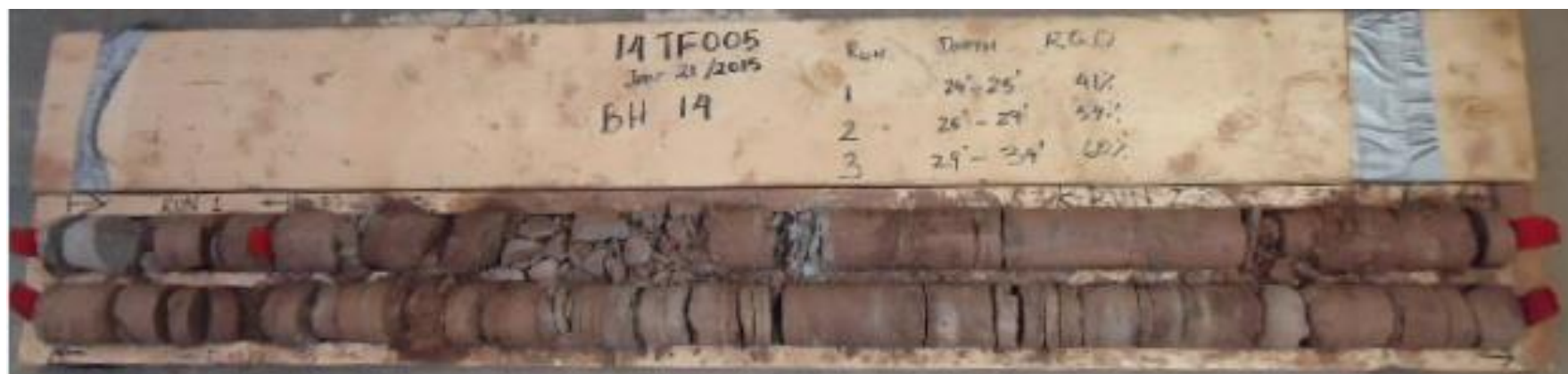
Photograph 2: Cores retrieved from borehole 14. Rock cores 1 to 3 from 7.3 to 10.4 m. RQD values ranged from 41% to 60%, indicating poor to fair rock quality.
