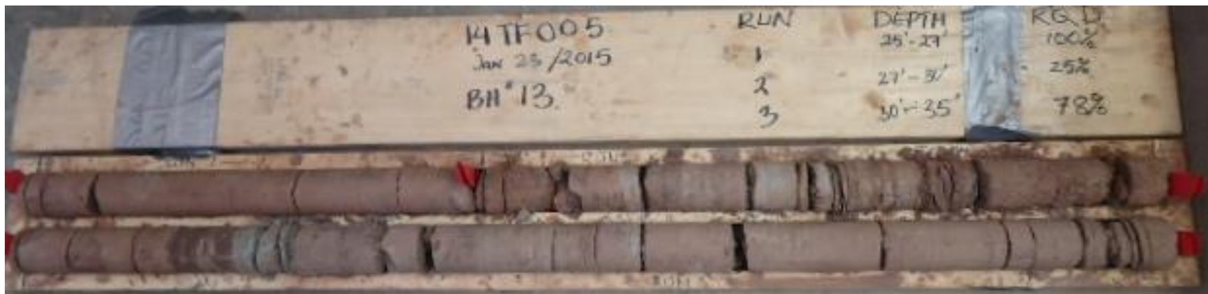
Photograph 1: Cores retrieved from borehole 13. Rock cores 1 to 3 from 7.6 to 10.7 m. RQD values ranged from 25% to 100%, indicating poor to excellent rock quality.
