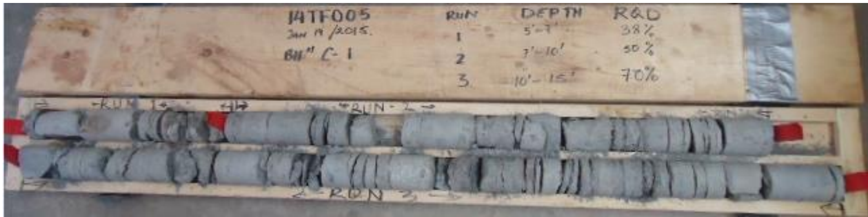
Photograph 1: Cores retrieved from borehole C-1. Rock cores 1 to 3 from 1.5 to 4.6 m. RQD values ranged from 38 to 70%, indicating poor to fair rock quality.
