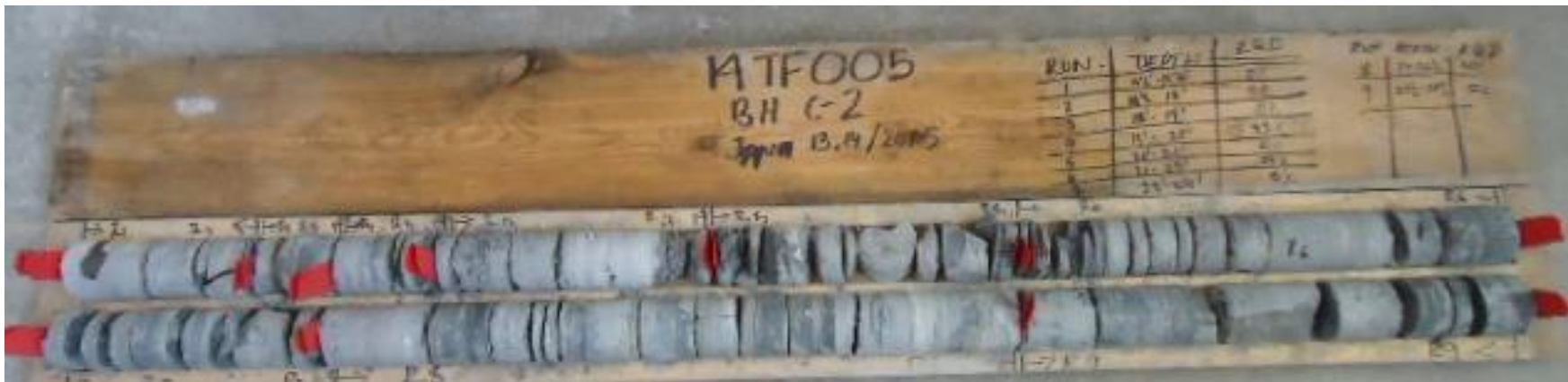
Photograph 2: Cores retrieved from borehole C-2. Rock cores 1 to 9 from 4.8 to 8.7 m. RQD values ranged from 0% to 50%, indicating very poor to poor rock quality.
