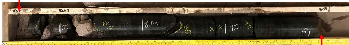
Borehole 18-6: Bedrock cored between depths of about 7.65 m to 8.55 m
