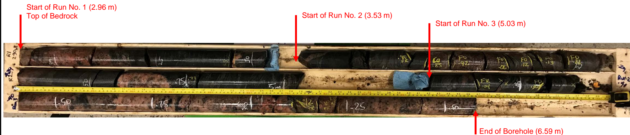
Borehole 18-1: Bedrock cored between depths of about 1.75 m to 5.73 m
