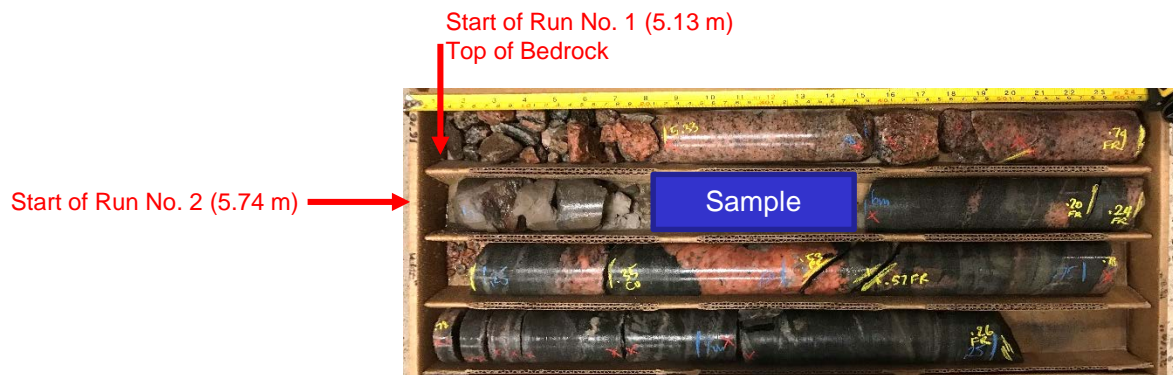
Borehole 17-7: Bedrock cored between depths of about 5.13 m to 7.26 m
