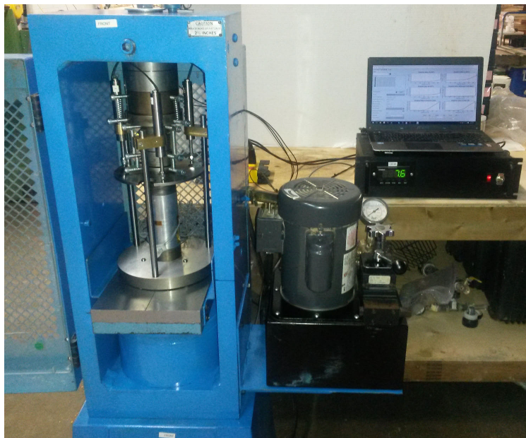
Figure 1: Forney loading frame setup for uniaxial compressive strength testing.
