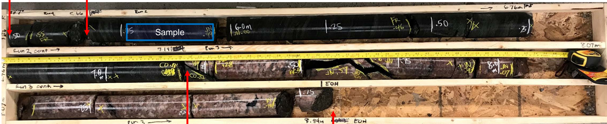
Borehole 18-8: Bedrock cored between depths of about 5.50 m to 8.84 m
