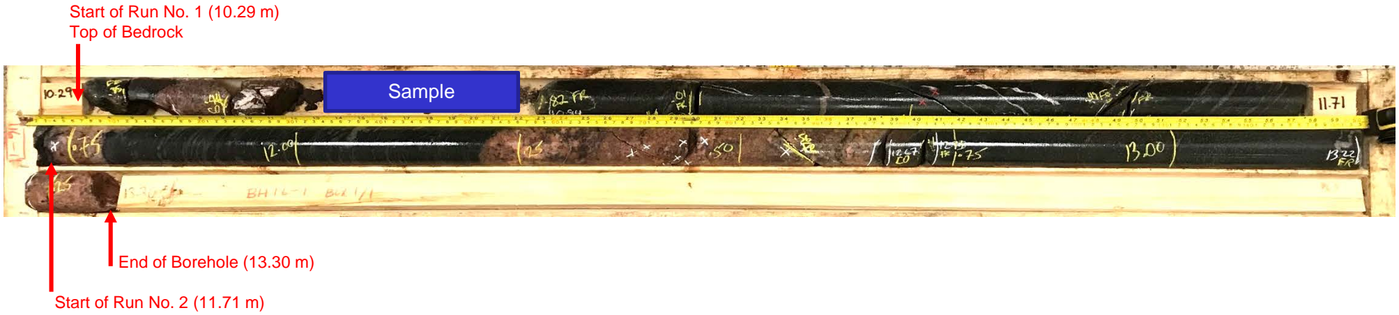
Borehole 16-1: Bedrock cored between depths of about 10.29 m to 13.30 m
