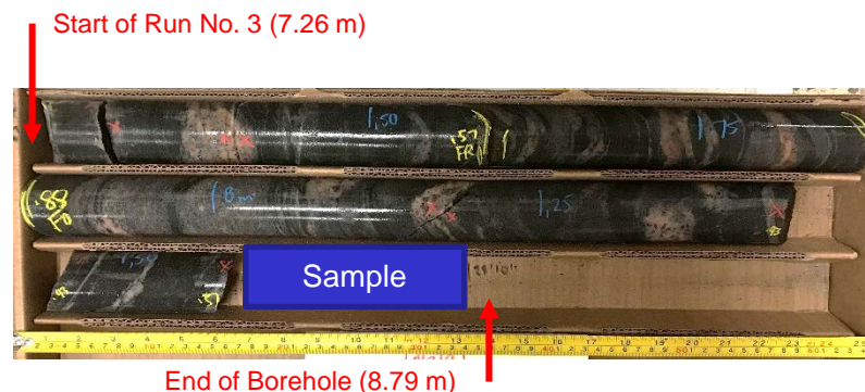
Borehole 17-7: Bedrock cored between depths of about 5.13 m to 7.26 m
