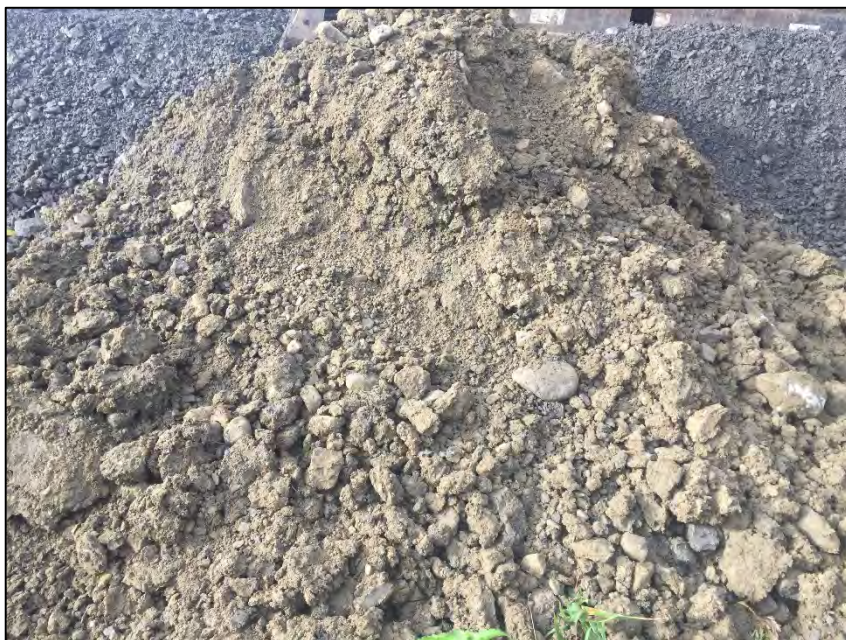
Photo B-8: View of sandy silt (fill) materials recovered from TP15-04 used to cover north TDA area.
