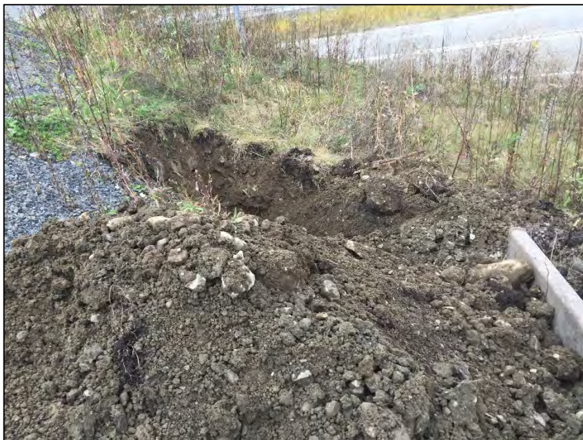
Photo B-16: View of gravelly sandy silt materials recovered at TP15-08 used to cover south TDA area.
