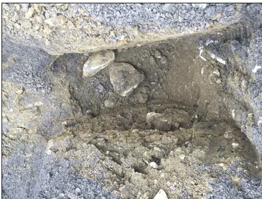
Photo B-10: View of sandy silt (fill) former road embankment materials recovered from TP15-05.
