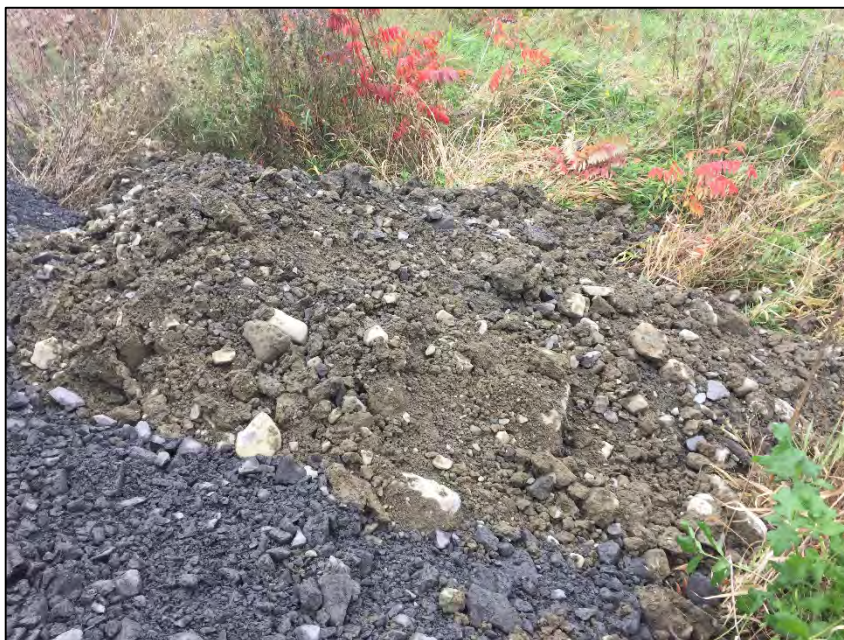
Photo B-6: View of silty sand (fill) materials recovered from TP15-03, representative of former road embankment materials.
