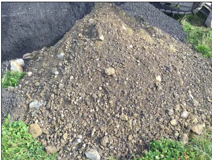
Photo B-14: View of silty sand (fill) materials recovered from TP15-07, representative of the former road embankment.
