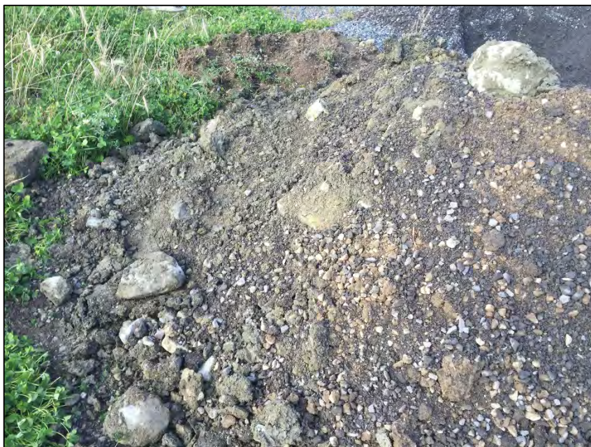
Photo B-20: View of sandy silt (fill) materials recovered from TP15-10, representative of the former bridge embankment materials.
