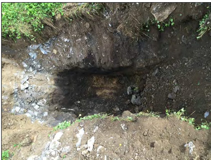
Photo B-24: View of open TP15-12 containing silty clay materials (fill).
