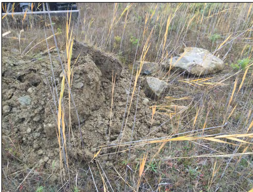
Photo B-4: View of silty clay (fill) materials recovered from 15-02.
