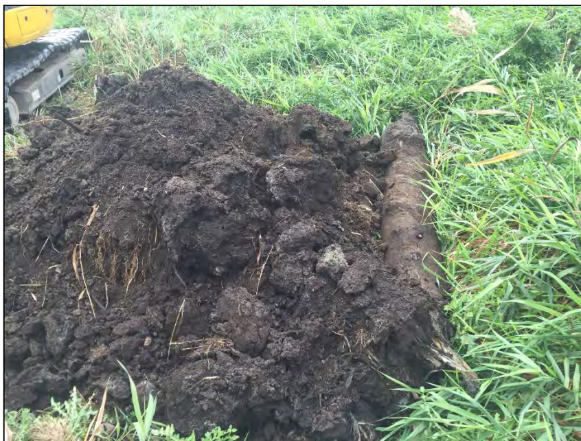
Photo B-2: View of amorphous peat fill materials recovered from TP15-01.
