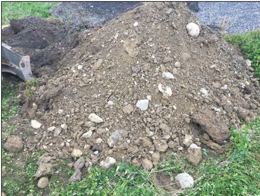
Photo B-22: View of silty clay (fill) materials recovered from TP15-11 used to cover the south TDA area.
