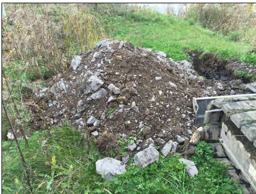
Photo B-18: View of silty clay materials recovered from TP15-09.
