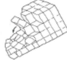
C) Toppling Failure
