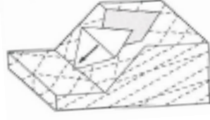
B) Wedge Failure
